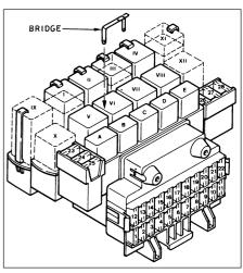
3.1c Component layout on the fuse/relay board. See Specifications for relay identification
